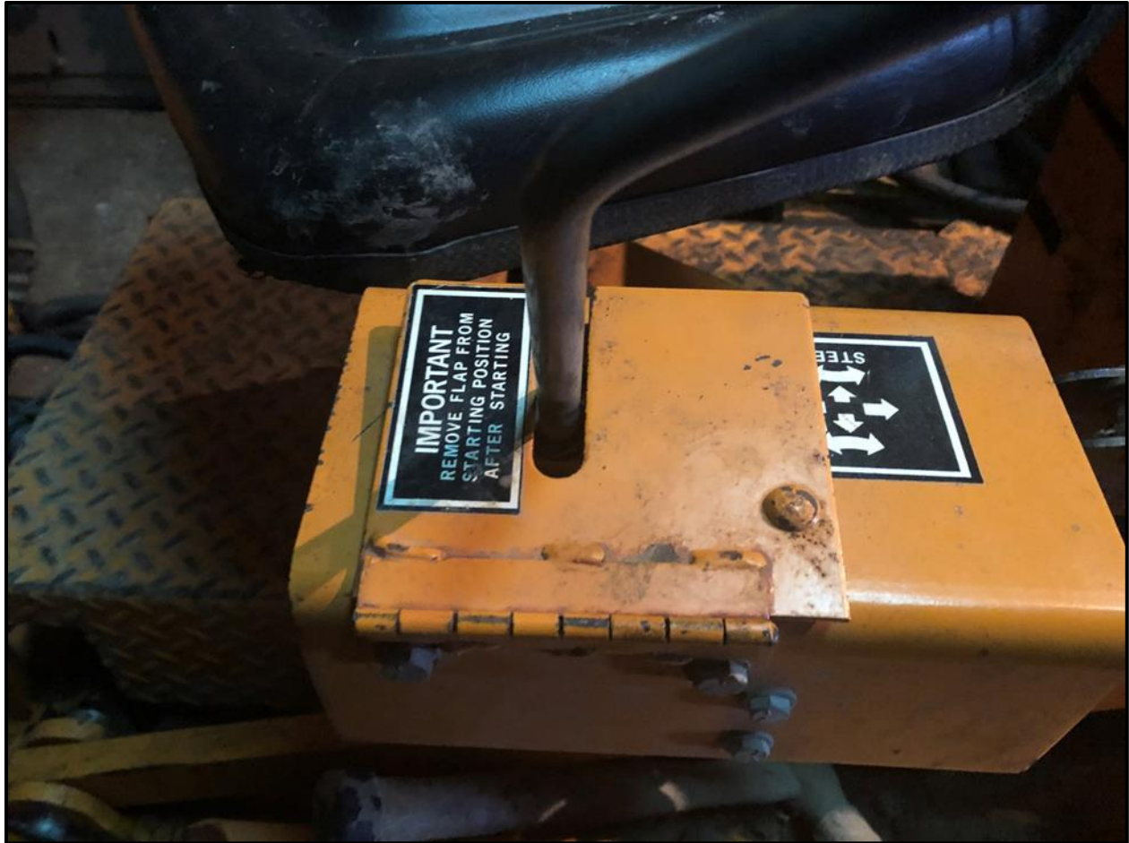
Figure 10 – Safety start latch in "start" mode.
