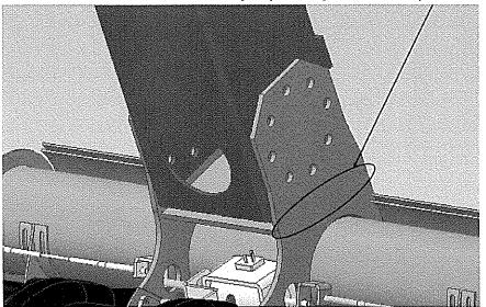
From between the ears, Inspect the top and bottom of the joint at both ends of the plate. Pay particular attention to the corners at the front and back edge of the plate.
